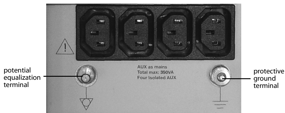
Figure C-4. Auxiliary power outlets.
